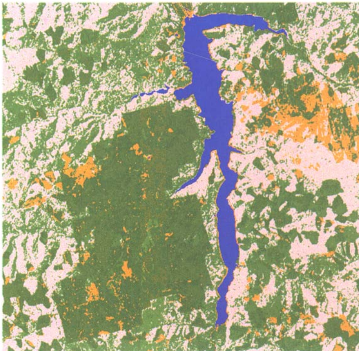
Plate 4. Classified subset of the Level 1A Scene in Plate 3. Spectral responses in the green, red, and NIR bands (layers 1, 2, and 3, respectively) are used to classify the scene. (Copyright CNES. Courtesy SPOT Image Corp.)
