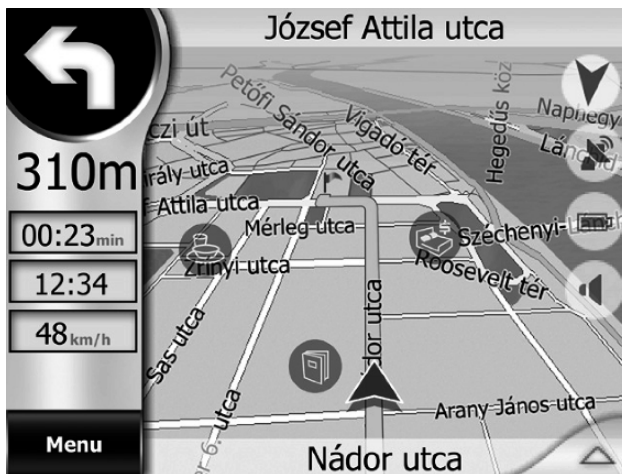
Fig. 12.8. Perspective views: maps are inclined to make it easier for users to match what they see in the display with their view in the real world. Source: iGO Website
