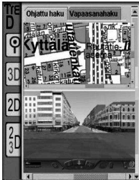
Fig. 12.9. Combining a 2D map of a urban environment with a 3D representation of what users see in the physical world to support navigation [28]. Image courtesy Ismo Rakkolainen, Tampere University of Technology, FI
