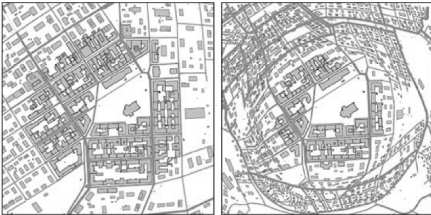
Fig. 12.5. Variable-scale maps: a circular area ( in the center ) is shown in full detail, while the remaining area is generalized and distorted to fit the available space [17]. Image courtesy Lars Harrie, Lund University, SWE
