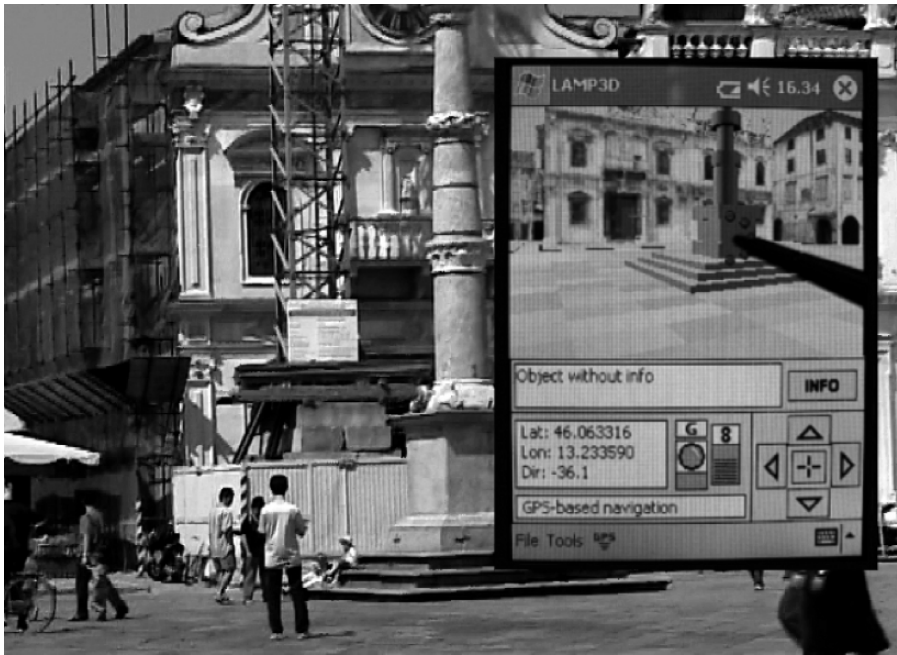
Fig. 12.11. In the LAMP3D system, the user selects objects with a stylus to obtain information on them [7]
