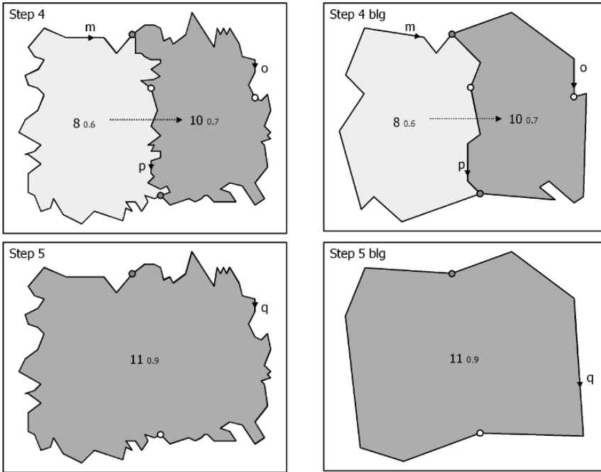
Fig. 5.5. Generalization example in five steps from detailed to coarse (see Fig. 5.4 for the first three steps)
