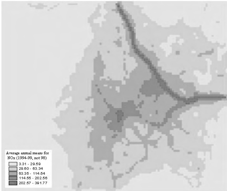
FIGURE 8.3A The average of the annual mean pollution levels, 1994 to 1999 (excluding 1998): NO x (µg/m 3 ).
