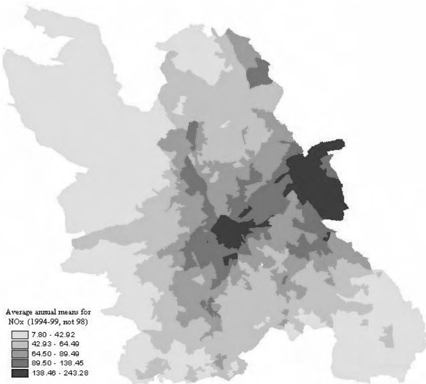
FIGURE 8.10 The NO x average of the annual mean pollution levels, 1994 to 1999 (excluding 1998) for Sheffield enumeration districts (µg/m 3 ).
