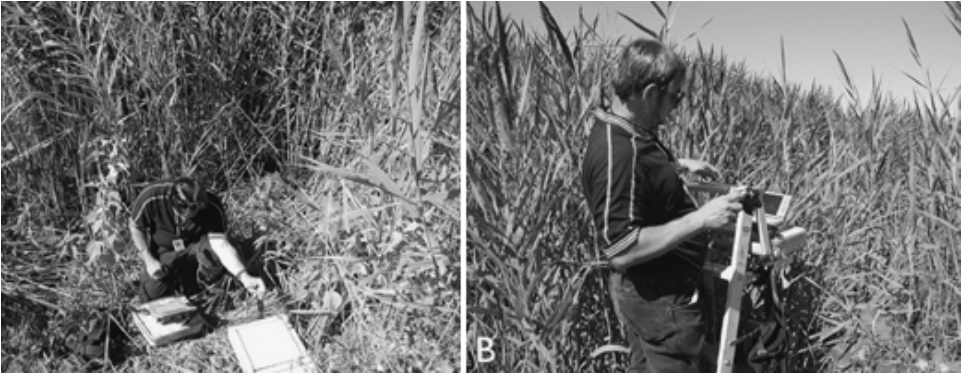
Figure 18.5 Field spectroradiometry sampling conducted August 14–17, 2001, at 4 of 13 wetland sites for comparison to the PROBE-1 reflectance spectra. The procedure involved recording (A) reference spectra and (B) vegetation reflectance spectra during midday solar illumination. Vegetation spectra were recorded from 1 m above the vegetation canopy.
