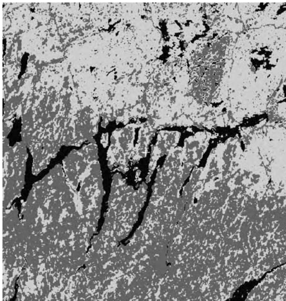
Figure 10.5 Land-cover classification of a portion of scene 17/29. Three classes are shown: water (dark), non-forest land (medium grey), and forest (white).
