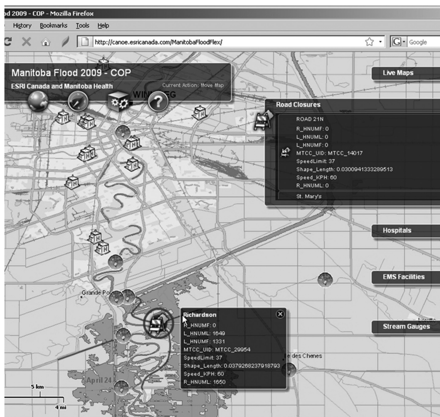
Figure 14.4 The common operational picture (COP) showed road closures to help identify the best evacuation routes.
