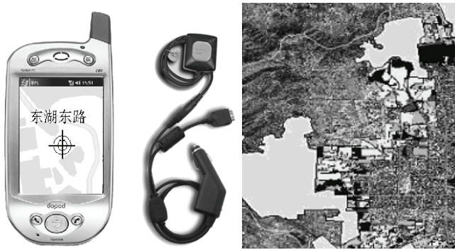
Figure 2.3. Mobile GIS for field data collection. (a) PDA hardware configuration for field data collection. (b) Land use maps and database from collected field data.
