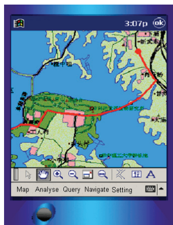
FIGURE 2.2 (a) The flood publishing software offers five functions, namely, map viewing, flood analysis and simulation, flood information querying, navigate to different monitoring sites and system calibration. Colour Figure 2.2 (b) Inundation map.
