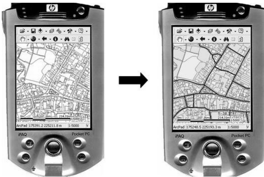
Figure 9.3. OSMasterMap ® data (Ordnance Survey © Crown Copyright. All rights reserved, 2005) displayed in an HP iPAQ using ESRI's ArcPad. The figure shows how appropriate symbolisation can enhance readability and usability of maps. Image on the left explicitly showing poor visualisation and image on the right displayed at the map specification guidelines for 1:5000 scale showing better data visualisation.
