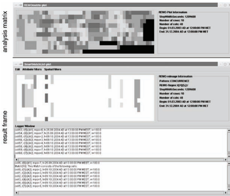
Figure 14.6. Porcupine Caribou case study. (Top) Analysis matrix for the motion azimuth of the caribou from Figure 14.1. Rows represent caribou individuals, columns represent time steps with an interval of two weeks. Eight azimuth classes are coded in greyscale, black refers to no data. (Bottom) Mined concurrence patterns of at least 5 individuals moving in the same direction. The found patterns correspond to northward spring migration and the southward autumn migration. The found motion patterns are highlighted in a results matrix and logged in the text frames below.
