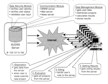
Figure 3.12 Software architecture of SUDSS prototype
