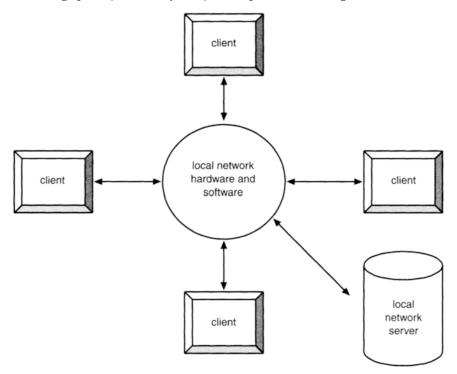
Figure 3.9 Local network server-based architecture for computerized support of same-place collaborative decision making environment
