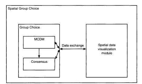
*Figure 3.10* Software architecture for Spatial Group Choice based on software module integration through dynamic data exchange protocol
