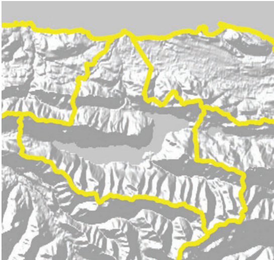
FIGURE 6.94 A hillshade map is a natural accompaniment to the basin delineation shown here. The hillshade is much too dark in its default form to allow other data to be seen on top of it. This hillshade was lightened by about 50 percent and the basin color was changed to yellow, which acts as a highlighter on the dark background.
