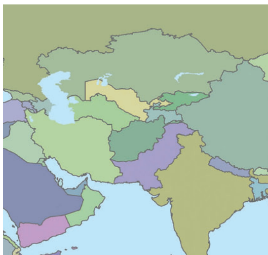
FIGURE 6.28 A very common way of separating political boundaries is to use different fill colors for each adjacent feature — making sure that no two adjacent features share the same color while also making sure that the colors all relate somewhat. In this map all of the colors are subdued cool tones. These kinds of political boundary maps make great background maps.
