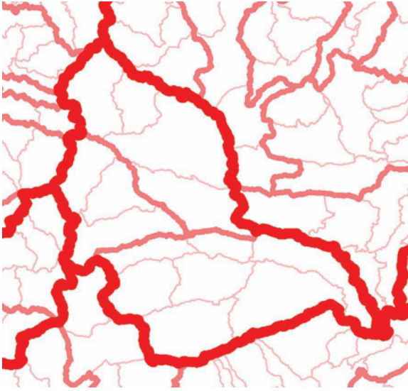
FIGURE 6.91 These nested basin levels are mapped with varying shades of red and varying line thicknesses. The smaller sized basins (sub-tributaries) are the lightest shade of red and the thinnest line. The medium-sized basins (tributaries) are a medium shade of red and a medium thickness line. The large-sized basin (mainstem) is the darkest shade of red and the thickest line. (This could be referred to as the porridge principle, a la Goldilocks.)
