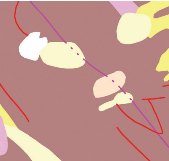
FIGURE 6.109 These geologic line features, shown in purple and red, are overlaid onto the geologic map units. The line features are bright since they can easily become lost within the colorful map unit polygons due to their small size. Line features such as the dikes shown here can be differentiated by their vertical location with dots to denote concealment and solid lines to denote surface dikes.
