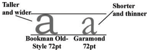
FIGURE 4.7 These two fonts show a wide degree of variation in height and width despite being the same point size.
