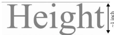
FIGURE 4.10 Point sizes are related to the height of the font as measured from the bottom of the lowest character to the top of the highest character. Not all fonts of the same point size will have the same height, though, as slight differences in character height exist between fonts.
