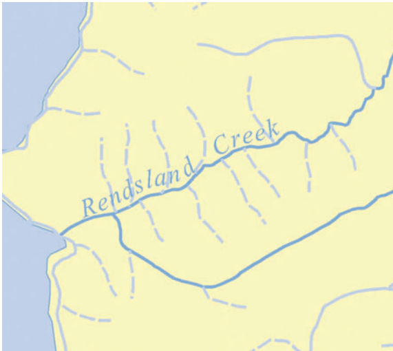
FIGURE 6.10 These stream lines have two different colors and two different styles according to their stream order. Both the ephemeral streams and major tributaries are the same color as the outlet water, but the ephemeral streams have a slight dashed pattern. The mainstem is a darker blue. The label text is splined and italicized, character spacing is wider than the default, space between “Rendsland” and “Creek” is also wider than normal. The label text color is the same as the outlet water color.
