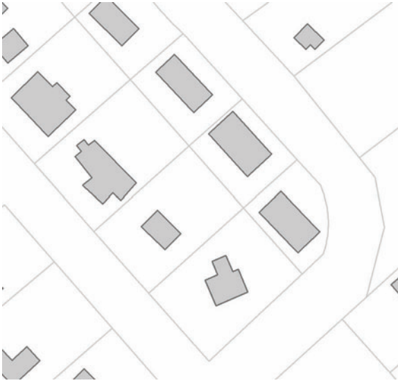
FIGURE 6.96 These gray building footprints are surrounded by lighter gray parcels. The parcel layer gives these buildings a lot more context, thereby adding to the viewer's understanding greatly.
