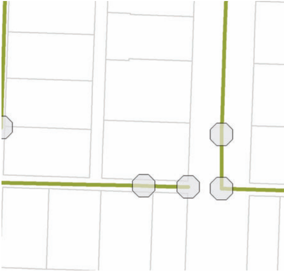
FIGURE 6.80 Transparent manhole symbols make the sewer main connections visible beneath them. The manholes are quite a bit larger in proportion to the rest of the map so that they are visible.
