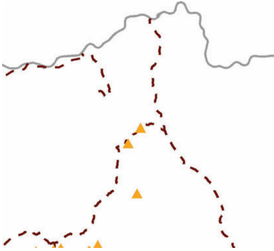
FIGURE 6.78 This trail map incorporates the nearby road feature and some campsite points. The solid gray line for the road and the dashed brown lines for the trails are intuitive symbols, as are the orange triangles for the campsites. This also illustrates the importance of ordering features correctly: campsites on top of trails, which are, in turn, on top of the roads. This allows everything to be seen without any loss of meaning.
