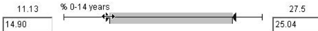
Fig. 4.88. A possible appearance of an element of Dynamic Query used for specifying constraints on the values of a single attribute
