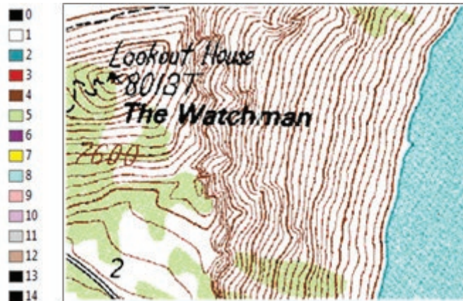
Fig. 2.18. An indexed-color raster stores a colormap that assigns a color to each value in the raster. Source: USGS
