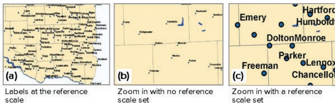
Fig. 3.16. (a) Text and symbols appear at their assigned size at the reference scale. (b) If the reference scale is not set, the symbols will always appear the same size. (c) If the reference scale is set, then zooming in or out changes the size of the text and symbols.
