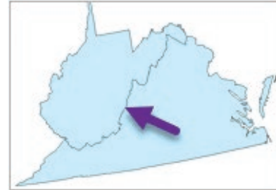
Fig. 1.5. A coincident boundary gets stored twice but is the same for both features.
