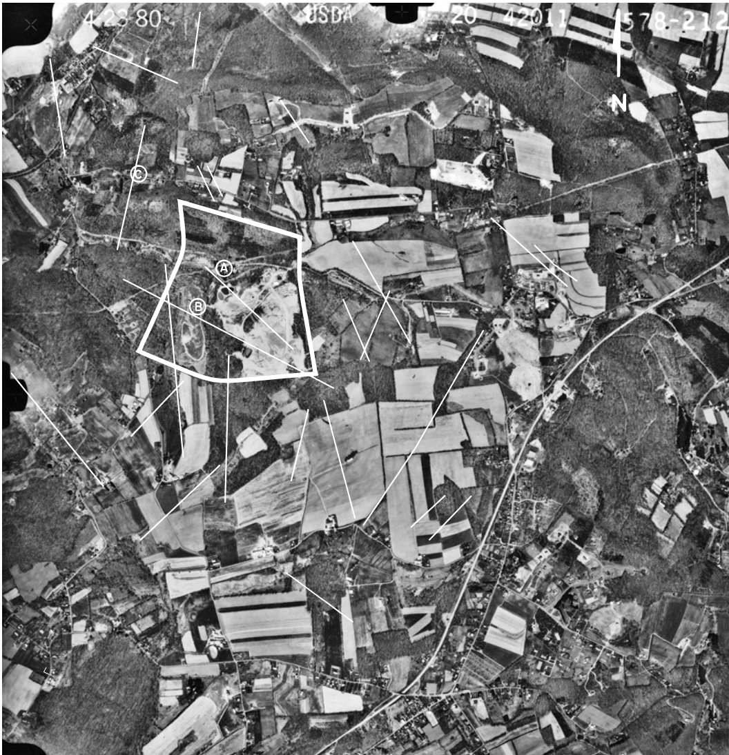
Figure 18.9a. Introduction. This fracture trace analysis presents findings based on the study of aerial photographs and geologic literature (see References) for the area on and around the landfill.
