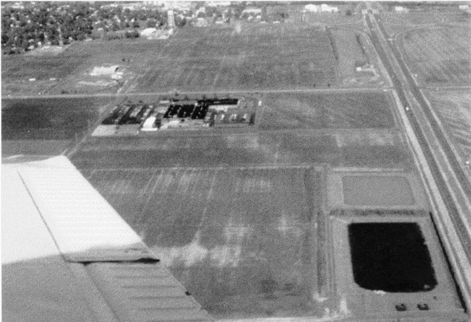
Figure 19.6. Low altitude aerial photographs of farm fields in Van Wert county showing wet areas, and the influence of subsurface drainage as lighter-toned linear features.
