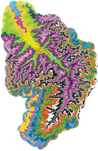
Figure 7.2. Digital elevation model of the Little Washita River Watershed overlain by TOPAZ-derived stream network. Each change in color on the DEM represents an elevation change of 7 m.
