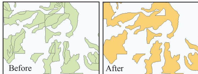
Fig. 10.11. A dissolve removes boundaries between polygons with the same attribute value, in this case, tree species.
