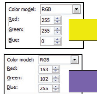
Fig. 4.16. Computers store and identify colors as mixtures of red, green, and blue light on a scale from 0 to 255.
