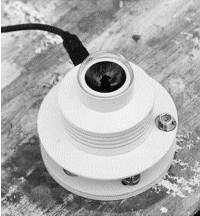
Fig. 4.9 Radiometer BIOMETER 501 installed at CIBA. Dpt. Applied Physics University of Valladolid (Credits: Calle 1997). Its spectral response to UV radiation is the proposed by McKinley and Diffey
