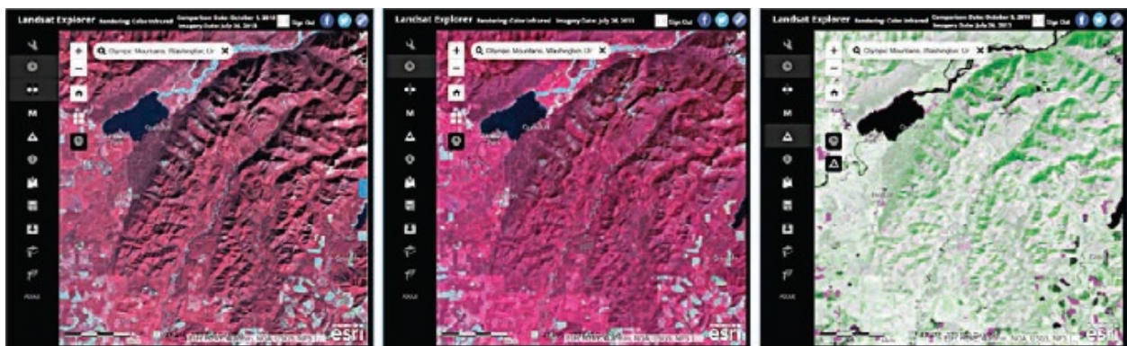
Figure 11.13. A change image of the Olympic Mountains in Washington showing how differences in sun angle can result in changes in spectral response that are unrelated to land-cover change. The figures show a comparison of imagery captured in 2010 (left) and 2013 (middle). The change image (right) shows a spectral difference (in green) on the north-facing aspects of the mountains that is caused by sun angle differences resulting from the 2010 image being captured in the fall,
