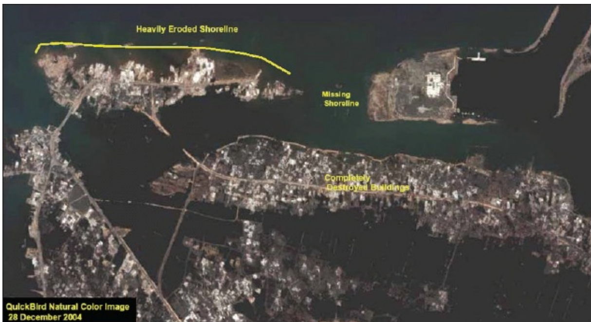
Figure 11.3. Single date change detection of the impacts of the 2004 tidal wave on Banda Aceh, Indonesia, as seen by DigitalGlobe's QuickBird satellite. Source: DigitalGlobe
