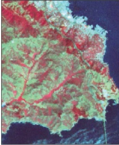
Figure 10.8. Unsupervised classification of southern Marin County, California. First, the image is sampled and then the sample pixels are iteratively grouped into clusters that are statistically similar.
