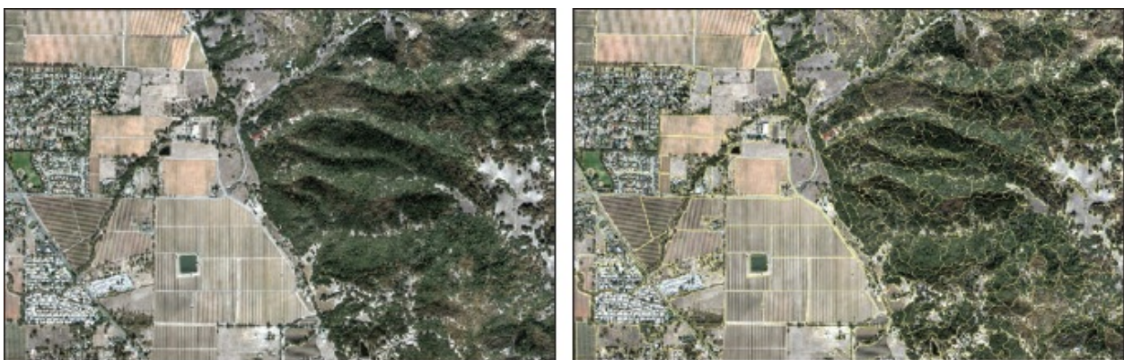
Figure 10.6. Example of image segmentation of six-inch high-resolution aerial imagery into objects that are outlined in yellow. Source: Sonoma County Agriculture Preservation and Open Space District
