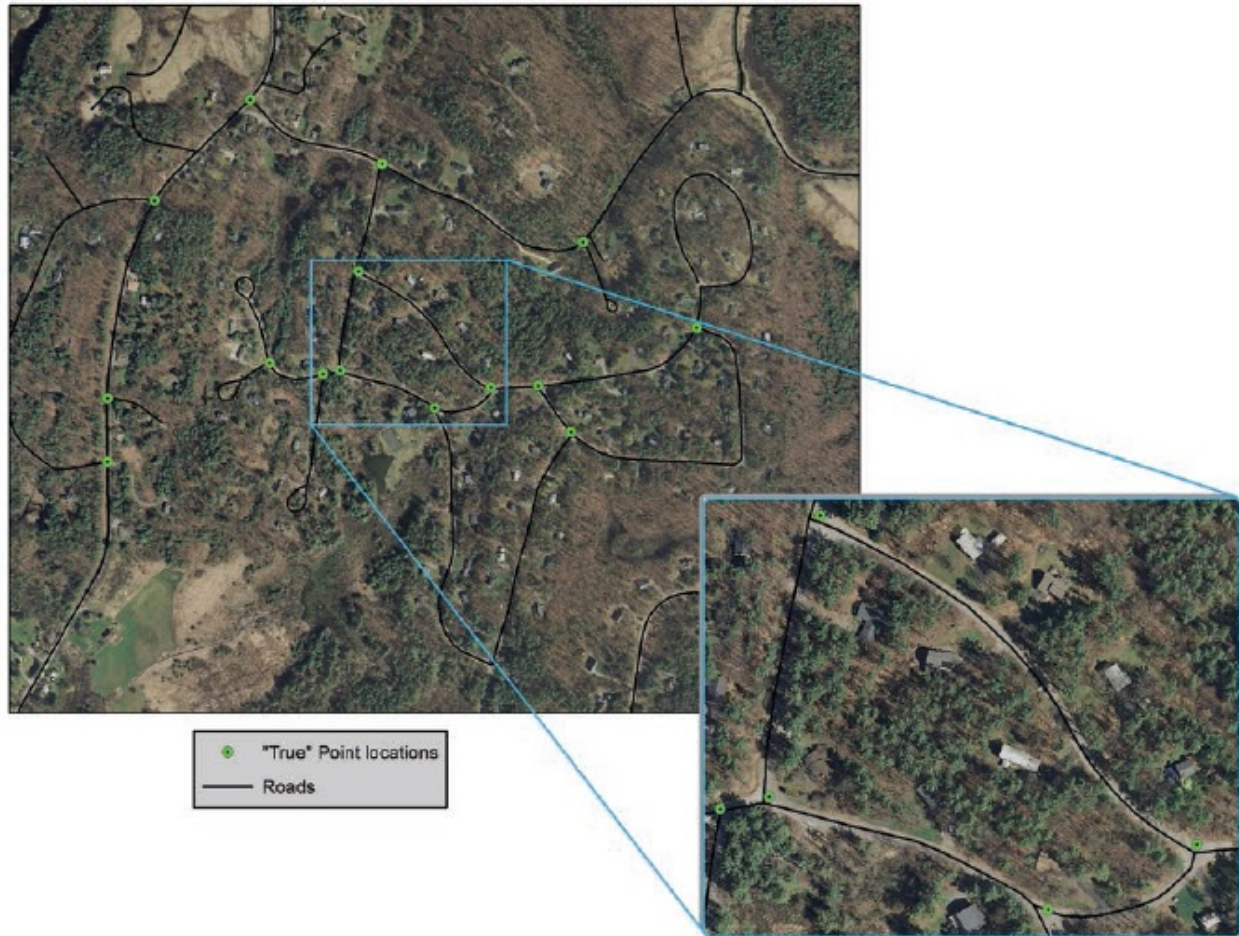
Figure 12.2. Example of positional accuracy assessment of a road network where the points on National Agriculture Imagery Program (NAIP) imagery show the surveyed ground location and the positional error in the geospatial road network layer
