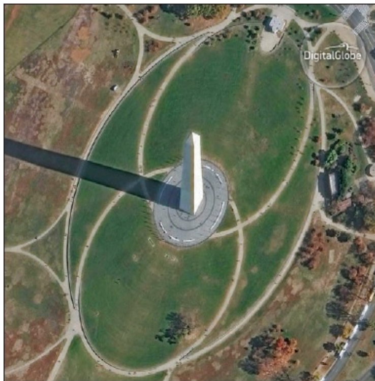
Figure 6.8. An image of the Washington Monument showing topographic displacement. Source: DigitalGlobe
