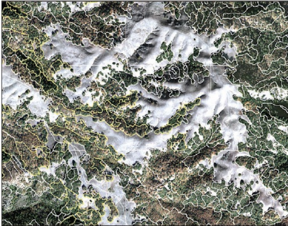
Figure 10.13. A segmented, high-resolution image with training sites shown as selected field-verified training sample objects outlined in yellow. Non-training site segments are outlined in white.
