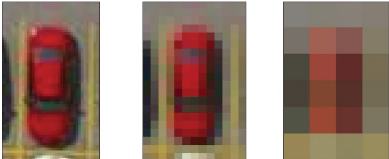
Figure 2.10. The impact of raster cell size on the level of detail depicted. The larger the cell, the less discernible detail. In this example a car is represented by three different image cell sizes but displayed at the same scale. The smaller the cell, the more information available to identify the rectangle of eight large reddish pixels on the right as a red sedan on the left.
