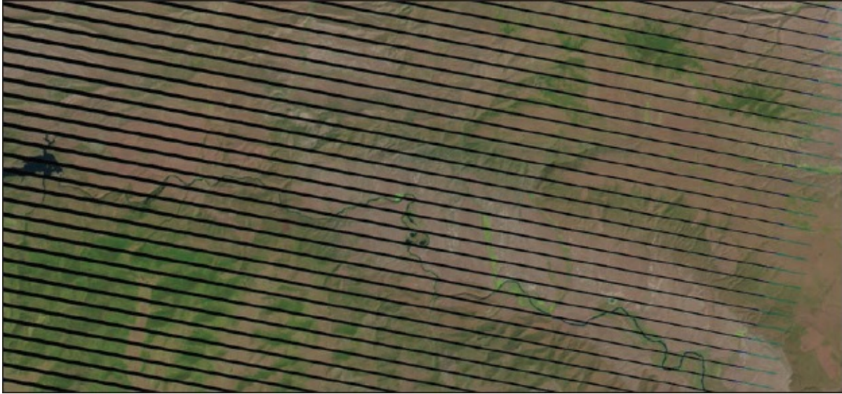
Figure 6.3. A portion of a Landsat 7 scene showing Scan Line Corrector gaps
