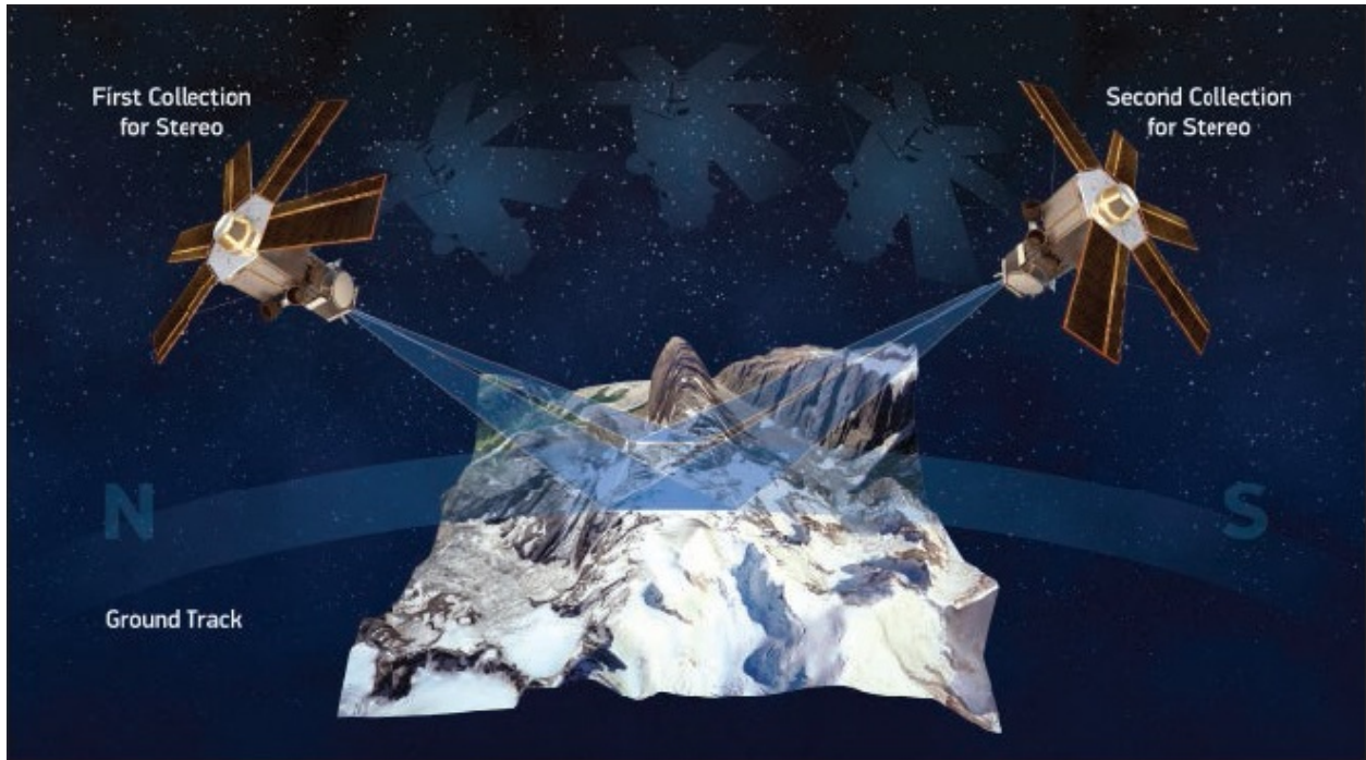
Figure 3.21. Diagram showing how pointable satellites can pitch from side to side during orbit to collect off-nadir stereo images. Source: DigitalGlobe
